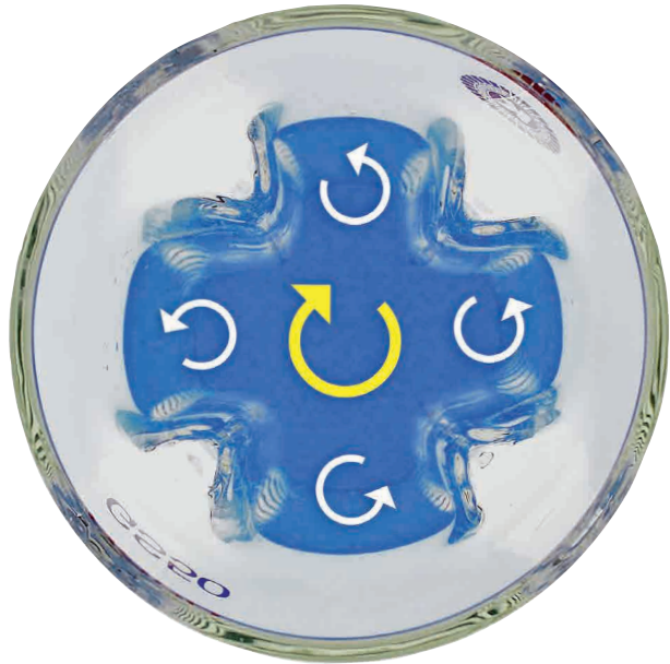
GS vessel principle (viewed from top)
